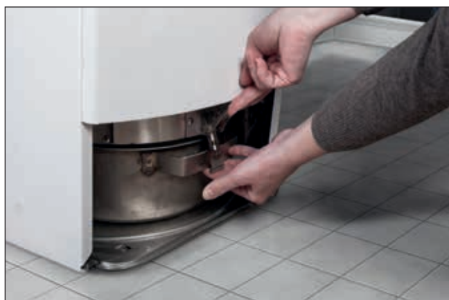
Open the hatch lock.
