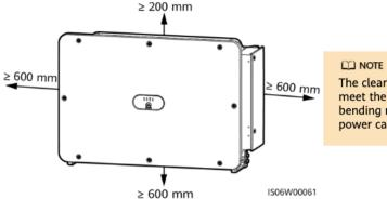
The clearance at the bottom must meet the requirements on the bending radius of the AC output power cable.
